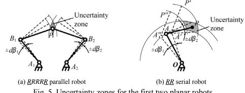
Fig. 5. Uncertainty zones for the first two planar robots.
