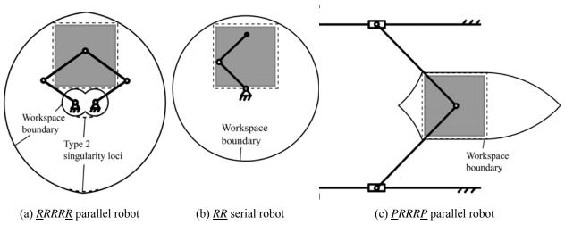
Fig. 4. Workspace of the planar robots under study (to scale).
