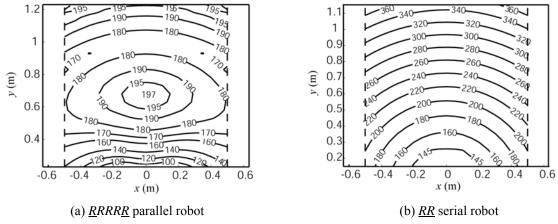
Fig. 6. Maximal position errors (in µm) in the desired workspace for the first two planar robots.
