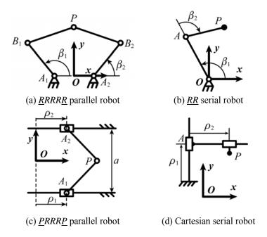
Fig. 1. The two pairs of planar robots under comparison (not to scale).
