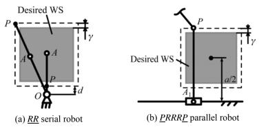
Fig. 2. Design constraints for obtaining the desired workspace.
