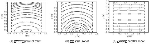
Fig. 8. Contour plots of the dexterity index for three of the robots over the desired workspace.
